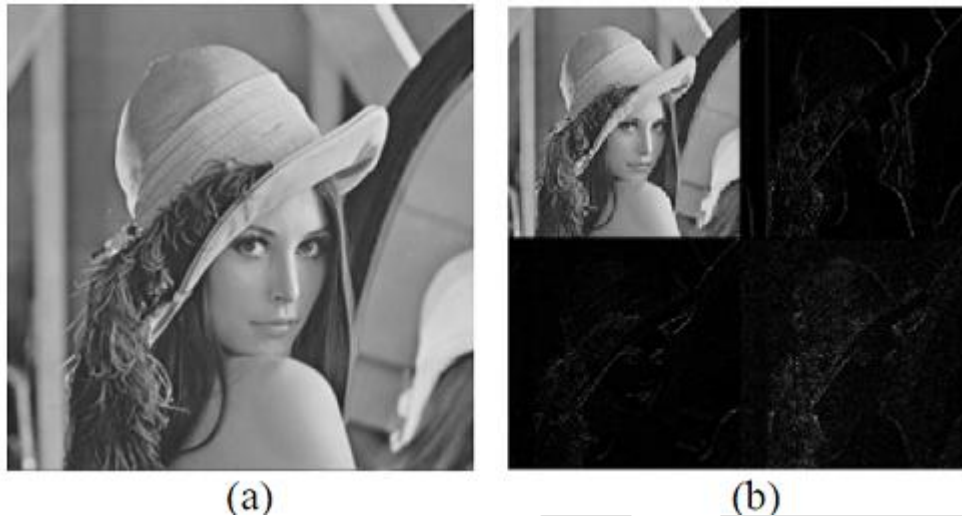
Figure 3. (a)Original image-Lena, (b) Result after the first-order 2-D Haar-DWT
